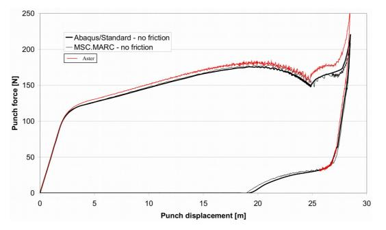
The results got into quadratic under-integrated without friction with the discrete formulation are in concord with the reference solution.
